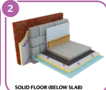
SOLID FLOOR (BELOW SLAB)
